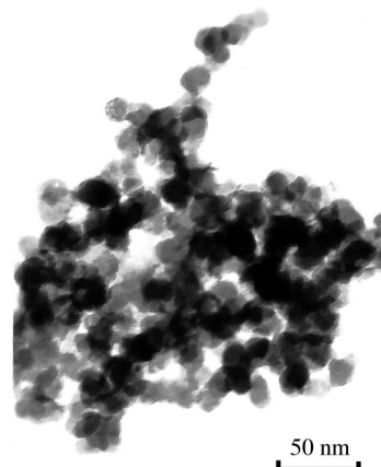
Fig. 2 TEM image of a typical sample of nanocrystalline \text{Cu}_{2-x}\text{Se} .
